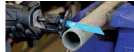
Bimetal Reciprocating Saw Blades: Metal Cutting
