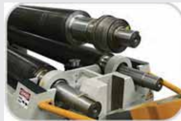
bending possibility of cones » setting for cone bending (standard)
