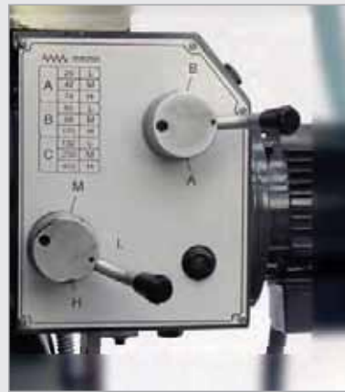
X- and Y-axes with 9 table speeds
