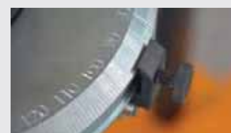
PIC: MANUAL SCALE WITH ANGLE SETTINGS (M MODEL)
