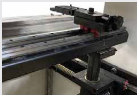
PIC: MOTORISED R-AXIS ON BACKGAUGE
