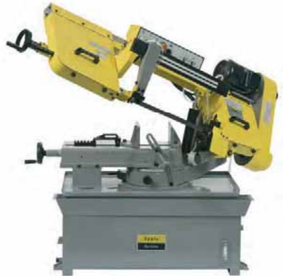
PIC: BS 230 VG WITH MITRE SWIVELING SAW BOW
