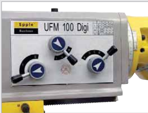
control panel for 11 spindle speeds
