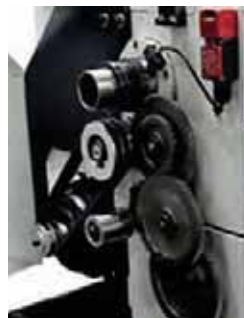
Frequency motor drive Fast shifting gears
