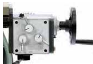
Automatic feed for the X-axis as standard (8 speeds)
