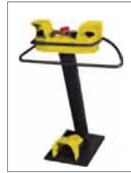
PIC: TWO-HAND CONTROL WITH FOOT PEDAL
