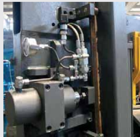
hydraulic blade tensioning
