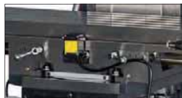
Precision grinding hardened table swivel from -45° to +45°
