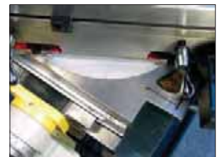
Cross Table rotatable by 45° to the left and right
