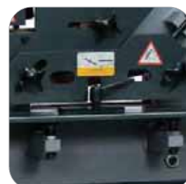
flat steel station table with angle stops and adjustable downholder
