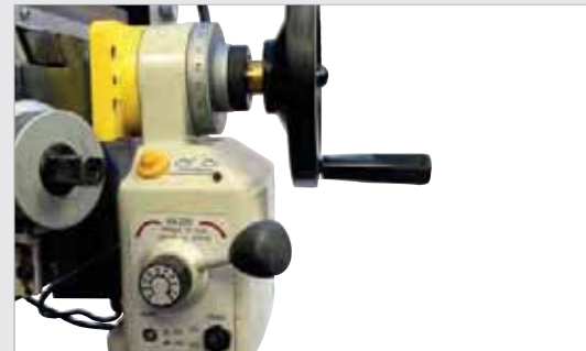
Y-axis with stepless feed control
