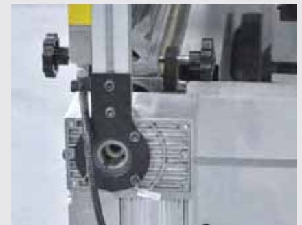
PIC: MOTORISED OR MANUAL CAMBERING OF THE BOTTOM KNIFE
