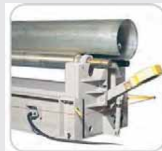
drop end » hydraulic drop end for rapid removal of the machined tubes (standard)
