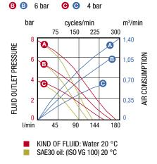
**Diaphragm pumps R. 1:1 for transferring,** made of die-cast aluminum, with black cataphoresis treatment that guarantees resistance up to 500 hours in saline fog.
