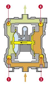
The slide valve of the air motor sends air (blue) to the left chamber which, pushing the membrane outwards, compresses the previously filled liquid (green). Through the effect of the pressure created valve 1 closes and valve **2** opens allowing the liquid to dispense
