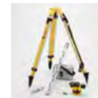
OLS 26, 8-part set (Art. No. 18460): OLS 26 optical level, BST-S construction tripod, TNL telescopic levelling rod, geo-folding rule, plumb line including line, rain protection, adjusting tools, carrying case.
